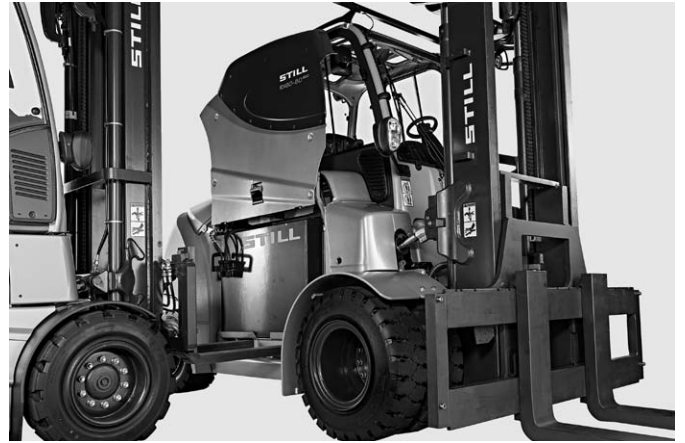
High availability thanks to fast battery changeover
