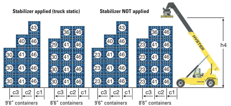
Note: All load centres c1, c2, c3 are taken from the front face of the (front) tyres, deduct 100mm for load centres taken from the front face of the Stabilizer.
