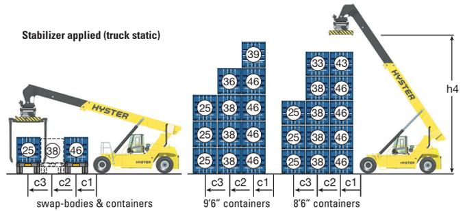
Note: All load centres c1, c2, c3 are taken from the front face of the (front) tyres, deduct 100mm for load centres taken from the front face of the Stabilizer.
