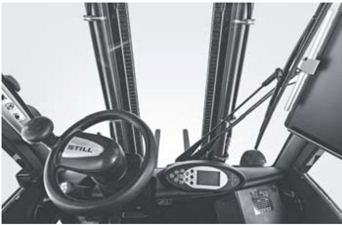
Excellent visibility looking forwards thanks to clear-view mast and low dash panel
