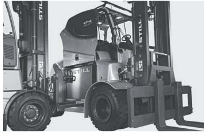
High availability thanks to fast battery changeover
