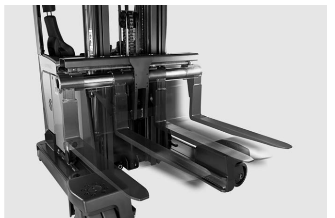
Hydraulic fork-spreading system ensures safe load handling
