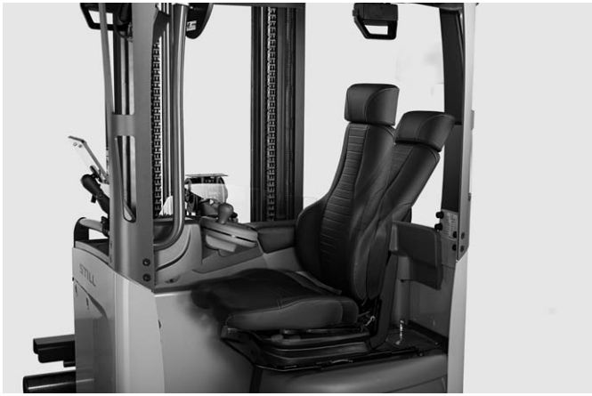
Comfortable tilt seat optimises upward visibility
