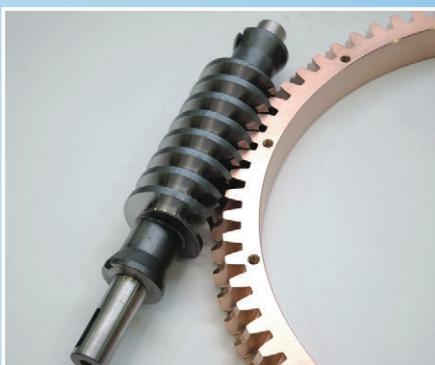
direct drive through worm wheel / worm gear
