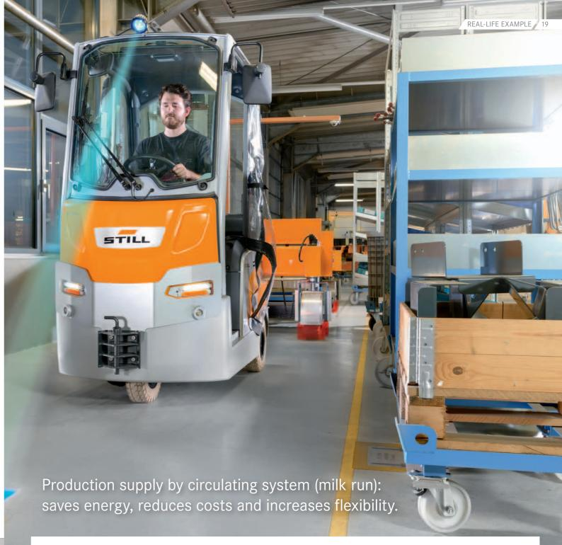
**The background:** The challenge was to switch a vehicle manufacturer's entire parts supply from front loader operations to a circulation system (milk run).
