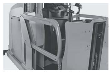
Tilting bar for ergonomic order picking to the last article on the pallet  $% \left\{ 1,2,\ldots,n\right\}$
