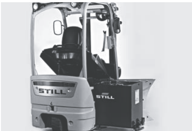
On-board battery bridge for lateral battery replacement using crane
