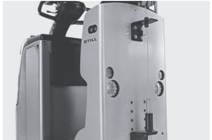
Fast coupling release from the driver's compartment
