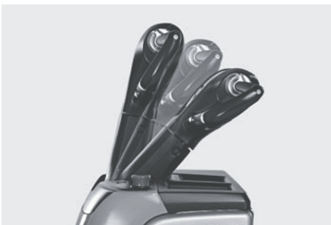
Height-adjustable steering for different drivers
