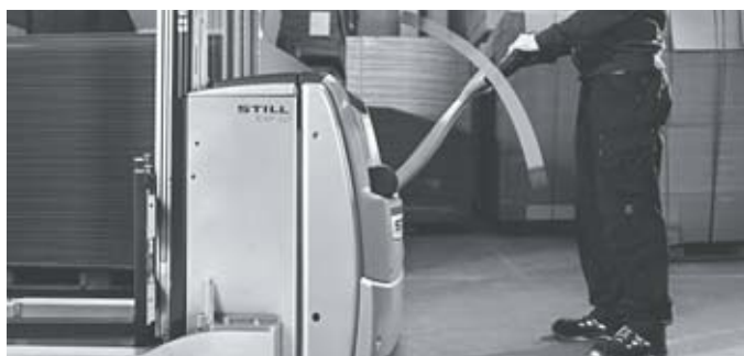
Safety in production: depending on tiller angle, speed is automatically adapted to the distance between the operator and the truck
