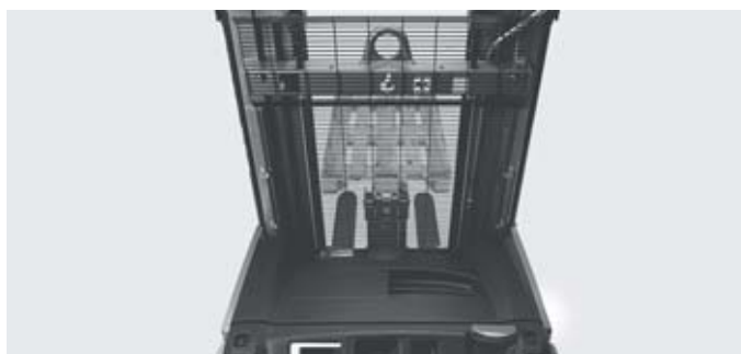
STILL free view mast always ensures the best view of the tips of the forks
