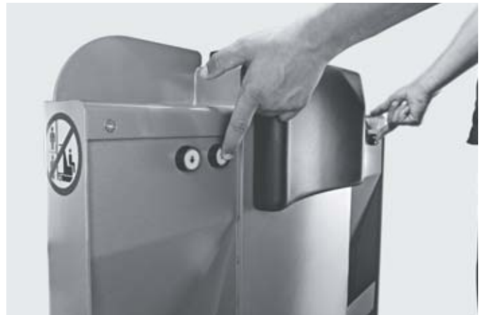
Safe two-hand operation of the auxiliary lift in the COP-L 07
