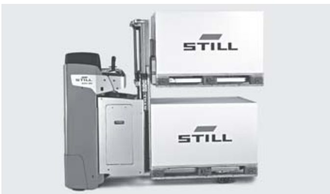
Also safe with two pallets: Use as double decker or high lift stacker
